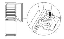
3. With the freezer compartment door closed, remove the crosshead screws from the lower door bearing and remove the door bearing downwards.
